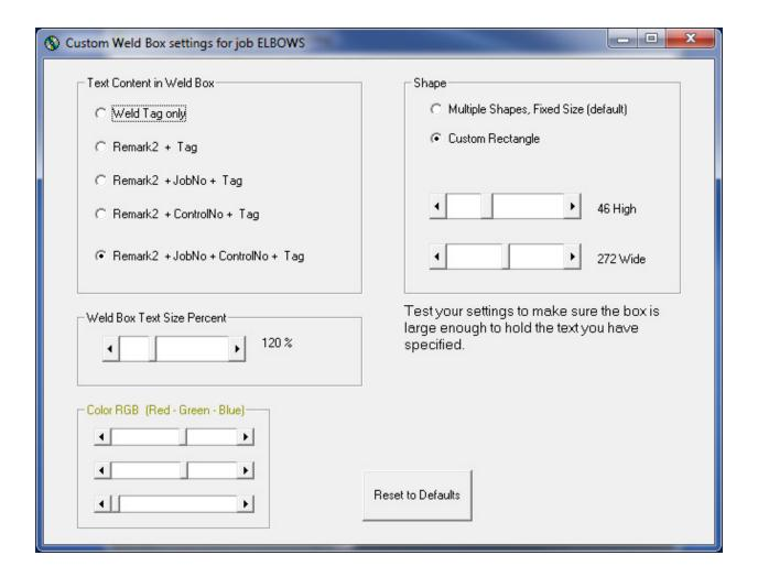
If you use any text content other than just the weld tag, you will likely need to select the weld box shape as Custom Rectangle in order to accommodate it. You can also change the size of the text and the color of the box. Note that these settings affect only the current job.
